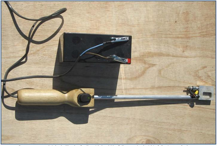
From my research it looks like the Oxalic acid should be fully vaporised within 2-3 minutes. Rather than having to disconnect the power by unclipping the battery connectors I decided to have a switch built into the handle. This makes the wiring assembly a bit tricky but should be a more elegant solution.
